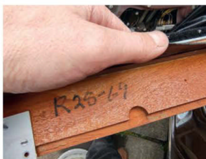
Numbers on the back of the door timber, tied to the car to ensure they all match.
