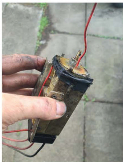
With the end plate removed, the plunger can slide out.
