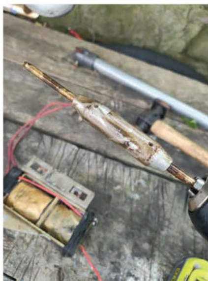
Spinning splunger in a drill allowed polishing, albeit to no avail.
