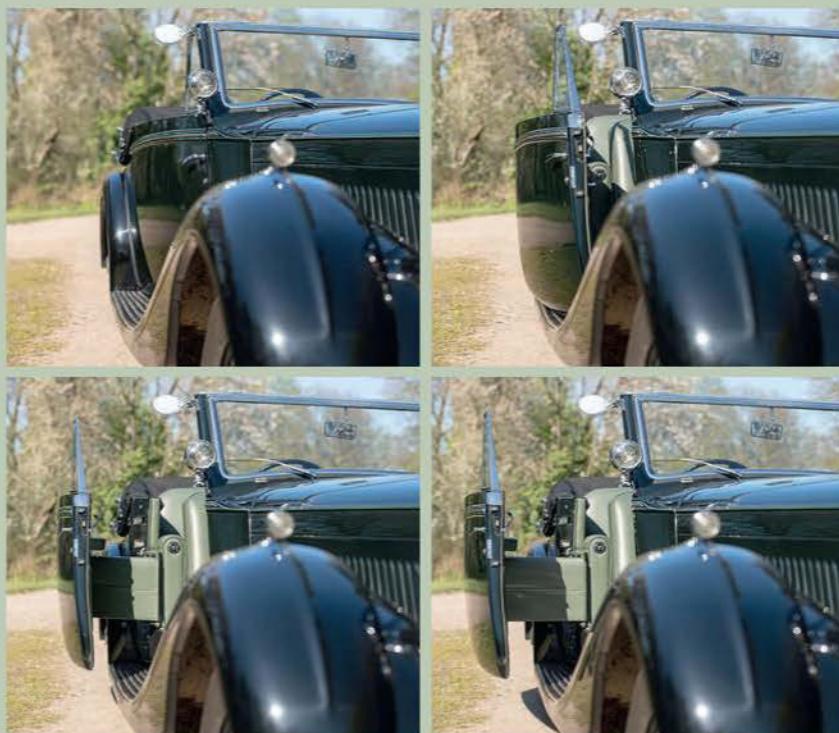
This ingenious design of door opening system is complex but eminently practical, particularly in tight spaces.
