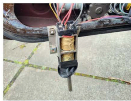
Testing the solenoid in situ by hanging it on a door card fixing hole.
