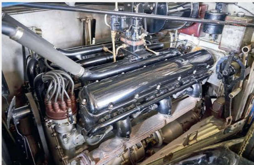
The 7.3-litre, 60-degree banked V12 engine, as used in the Spectres and subsequent Phantom IIIs.
